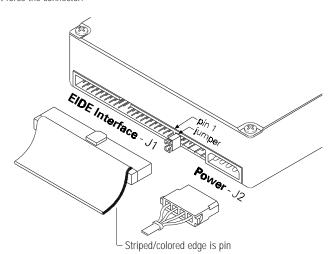
After attaching the IDE interface cable and the power cable to the Maxtor hard drive, verify that all other cables connected to other devices, the mother board or interface card(s) are correctly seated.
