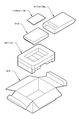
Figure 4 - 2 Single Pack Shipping Container (Option A)
