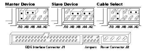
Before installing the drive in the computer, you **must** determine how the jumpers on the Maxtor hard drive are to be set for your system based upon the use of the Maxtor hard drive as either a Master or Slave device. Maxtor hard drives are shipped with the Master jumper setting enabled.
