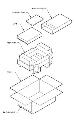
Figure 4 - 3 Single Pack Shipping Container (Option B)
